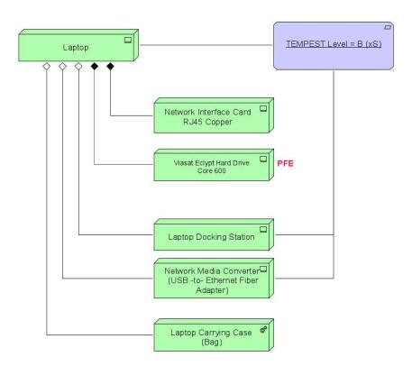
Figure 1: End-user Laptop Breakdown
