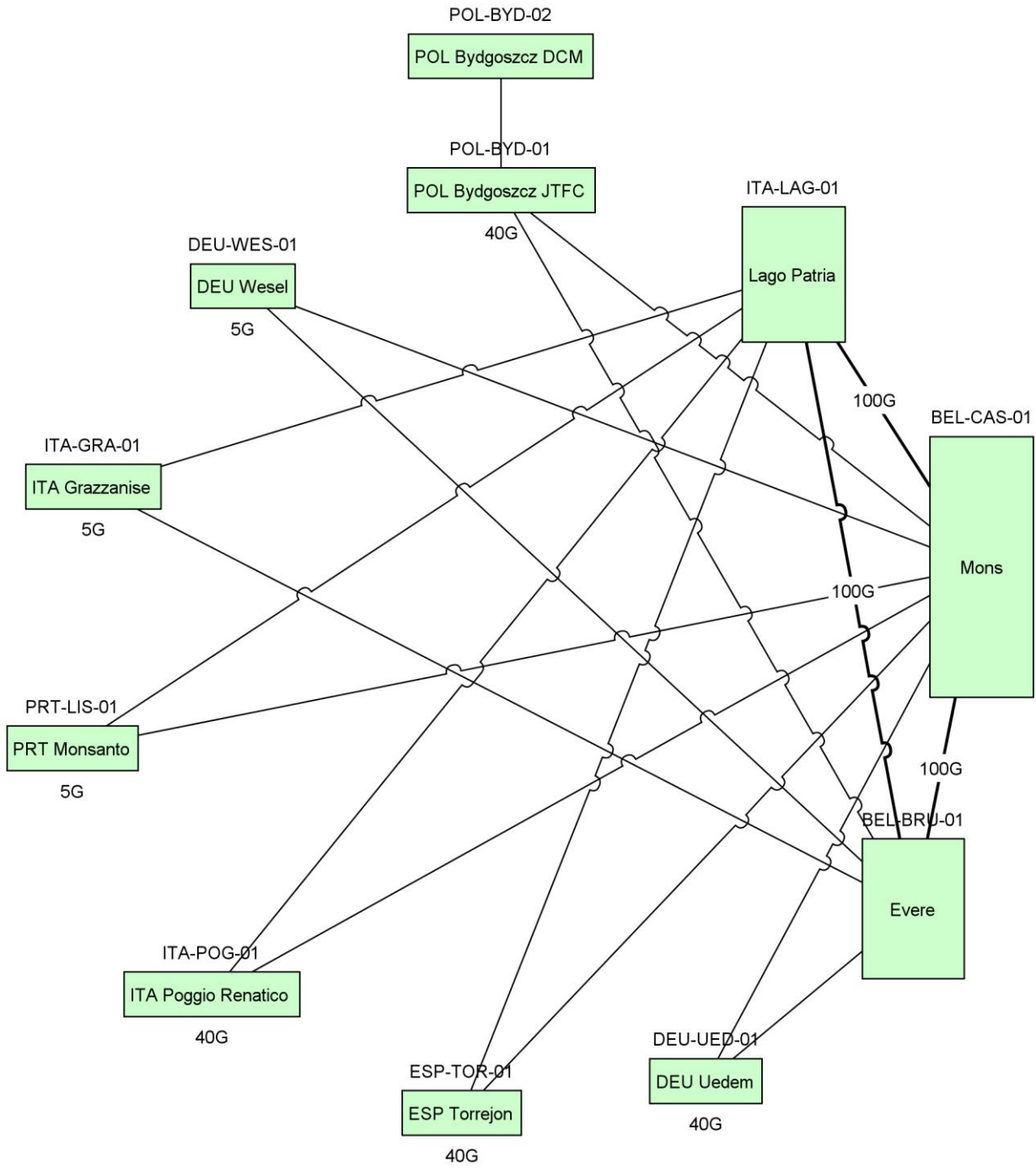
Figure 3-16 Standard Node network topology – Transport Perspective
