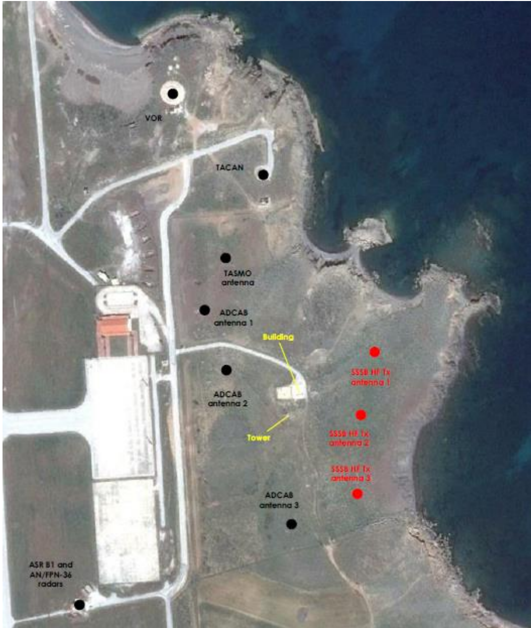
Figure 4: HF-TX Site Kartisinoudi (Skyros Island) – Current Site Configuration
