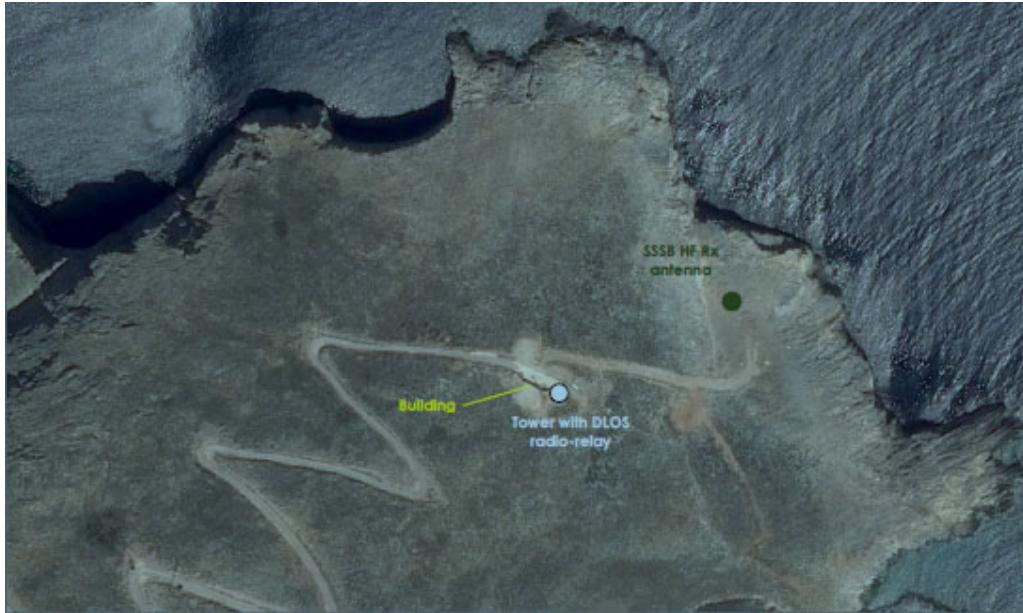
Figure 5: HF-RX Site Limnonari (Skyros Island) – Current Site Configuration
