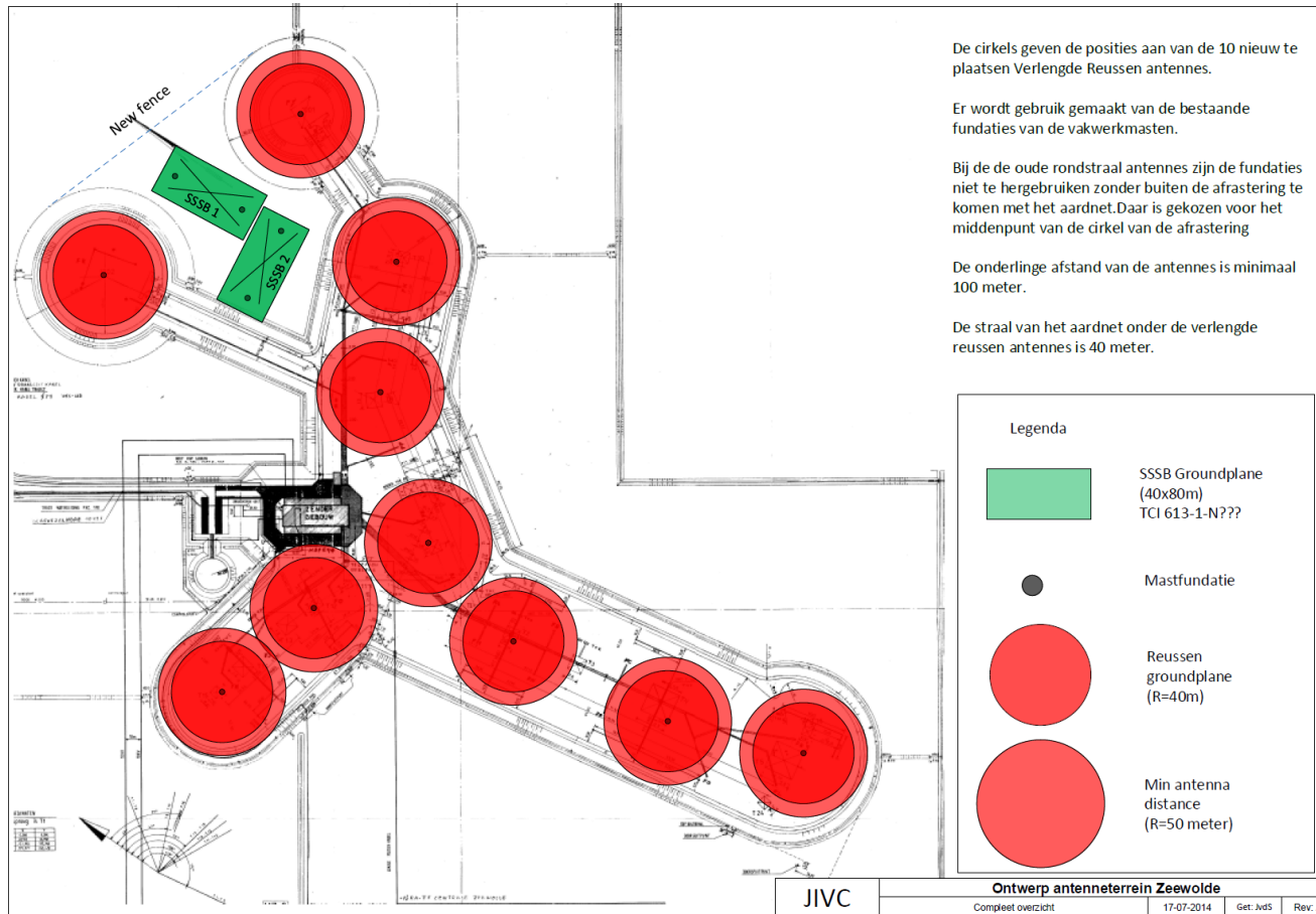
Figure 7: HF Rx Site Zeewolde Location, The Netherlands
