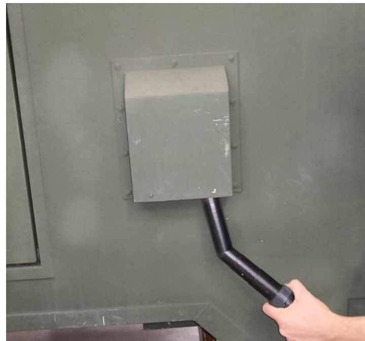
Figure 3.2.2.2-2 Cleaning GPFU Air Intake on Dismounted Container
