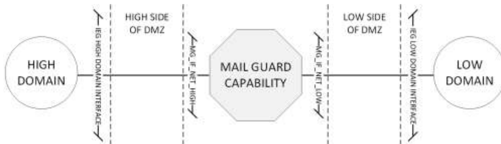
Figure 22: MG in DMZ Architecture: Domains and Interfaces
